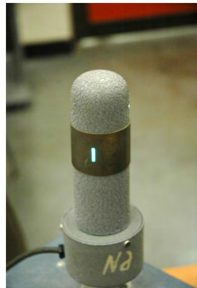
The Hydrogen-Deuterium light source is used with an external high voltage (5000 VAC) power supply. All electrical contact points are insulated, but care should be exercised in its use, and the power supply should always be turned off before handling the source lamp. This source will be used for taking the actual experimental data. **Be sure to turn on a fan aimed at the lamp.** Otherwise the tube will overheat and the line emission intensity will drop.
